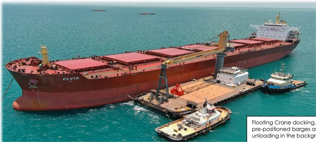
Floating Crane docking, with pre-positioned barges awaiting unloading in the background
