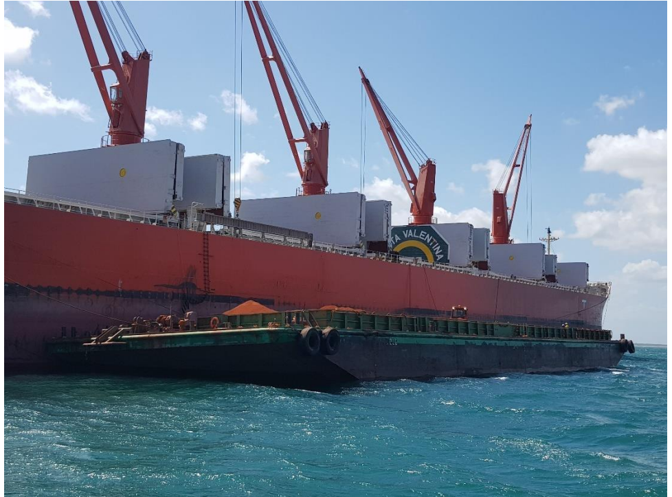
Figure 6. Transshipping – barge alongside ~60kt Supermax vessel
