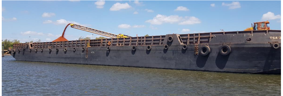
Figure 5. Barge loading (new large 7kt capacity dumb barge)
